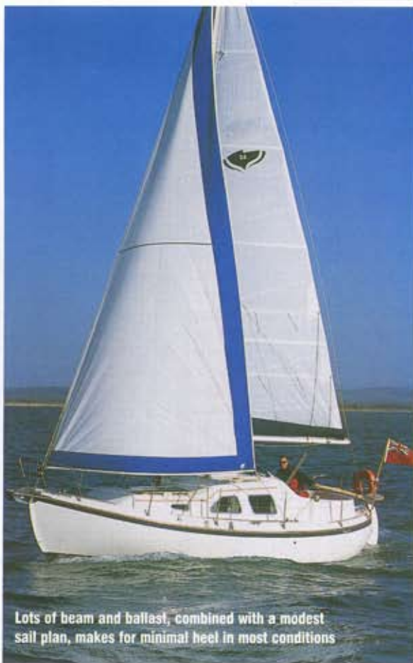
Built since 1980, the Midget has changed little; the bowsprit and the seats in the stern rail are among the few additions
